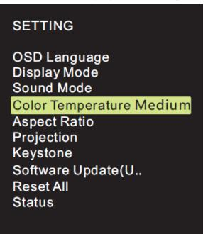
3. Press ( and ) buttons to select the desired Color Temperature mode.
