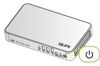
5. When "Power off/Please press the power button again" message appears, press of power button. The projector will turn off.
